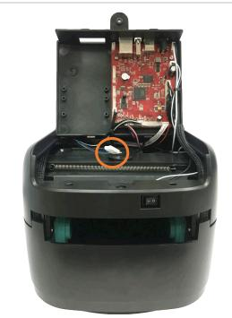
6. After opening, pull out the wire just put into the hole and insert it into the wafer 1x10P on the main board.
