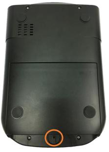
5. After closing the upper cover, turn the printer upside down, remove a screw located on the bottom cover, and open the bottom cover.
