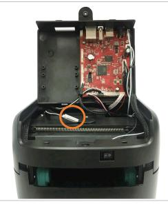
After opening, pull out the wire just put into the hole and insert it into the wafer
